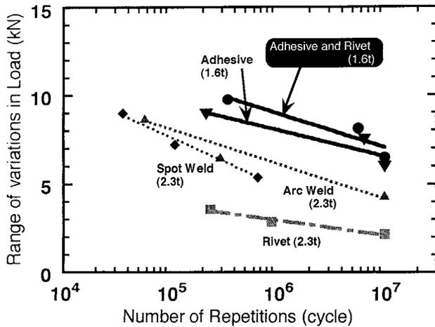
Fig. 7. Comparison of fatigue strength of the various kinds of joints.
