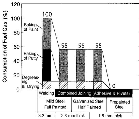
Fig. 10. Change of consumption of heating fuel gas used in the painting process of enclosure factory.
