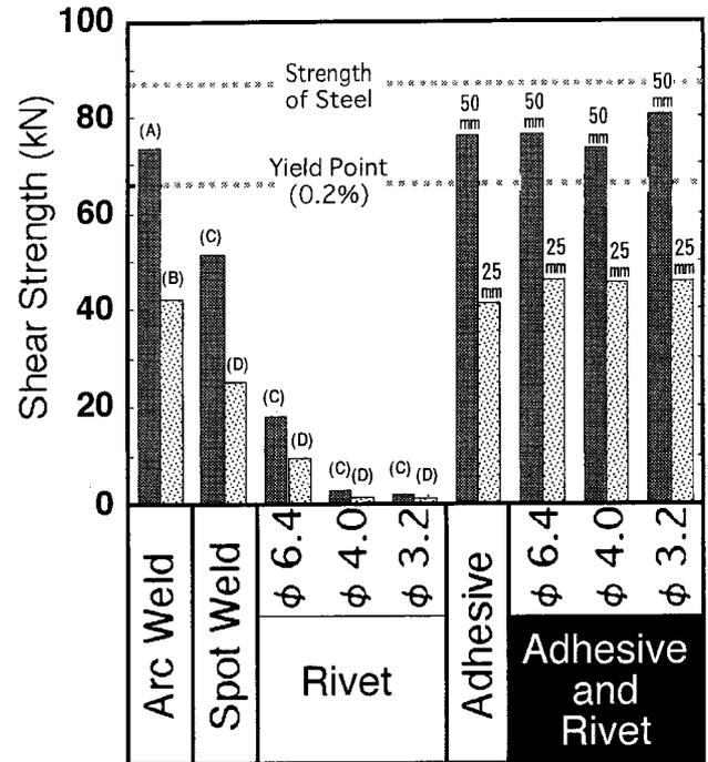
Fig. 5. Comparison of the shear strength between arc welding, spot welding, rivet, adhesive and the combined use of adhesion and rivet (substrates: 2.3-mm-thick cold-rolled steel).
