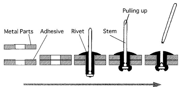
Fig. 3. Schematic illustration of the joining process used for adhesive and rivets.
