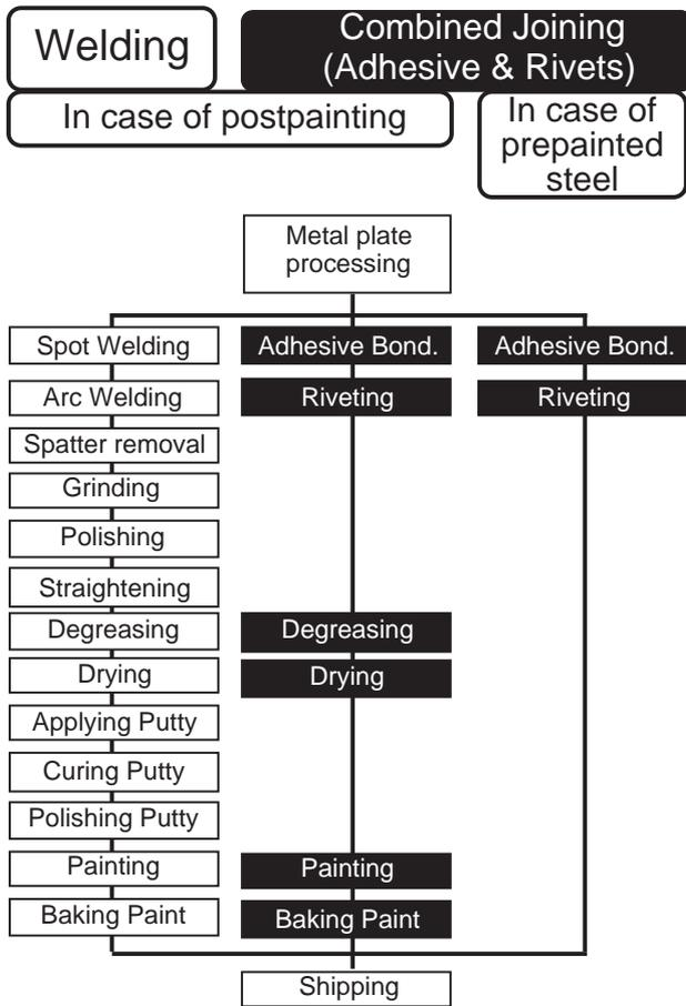
Fig. 4. Comparison of manufacturing process between welding and the combined use of adhesive and rivets.
