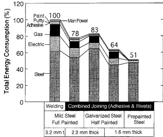
Fig. 11. Change of total amount of energy consumption from mining iron ores and crude oil to completion of enclosure assembling.
