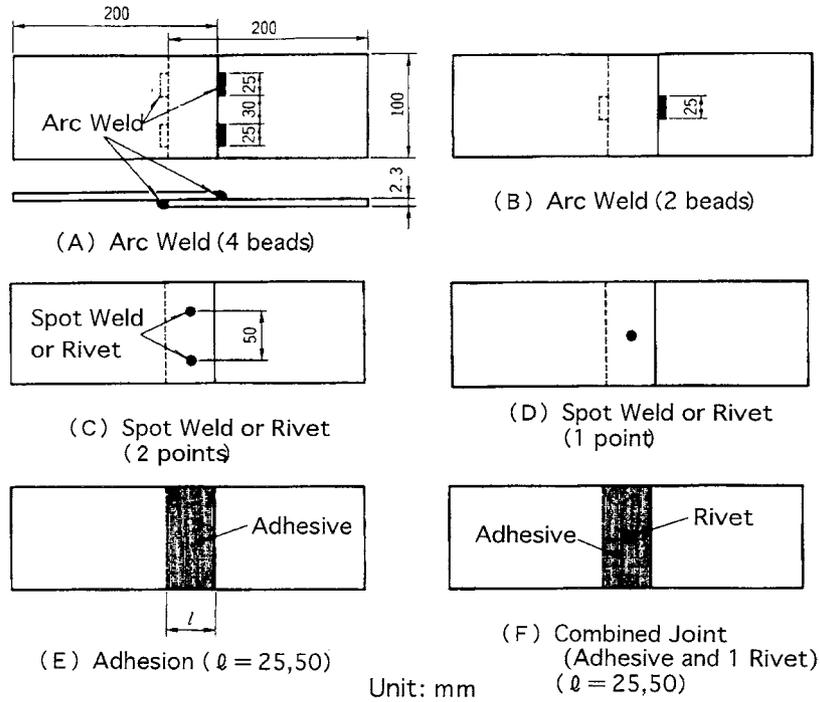
Fig. 6. Types, shapes and dimensions of test pieces.
