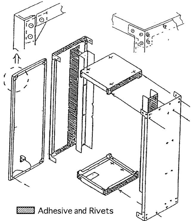
Fig. 2. One example of control panel enclosures assembled by the combined use of adhesive and rivets (800 mm  $W \times$  800 mm  $D \times$  2300 mm  $H$ ).
