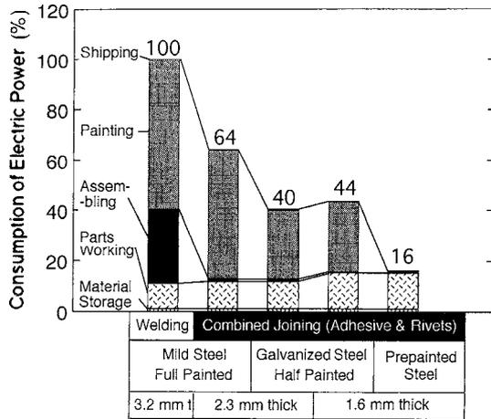
Fig. 9. Change of consumption of electricity in manufacturing process of an enclosure.
