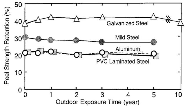
Fig. 8. Results of outdoor exposure tests of adhesion upon various adherents.
