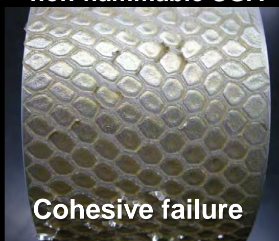
Fig.19 Condition after fracture
