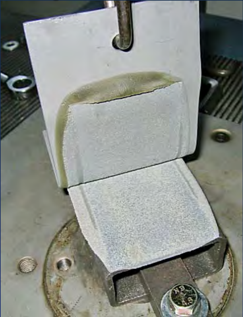
Fig.11 Cohesive failure (example)
