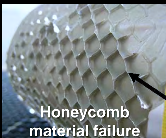
Fig.19 Condition after fracture
