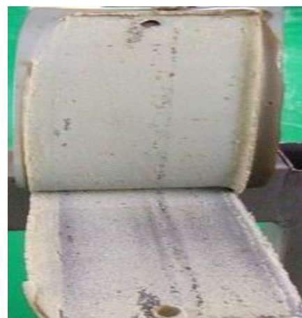
Fig.2 Appearance of fracture mode on oily mild steel surface.Excellent cohesive fracture is seen over all areas.
